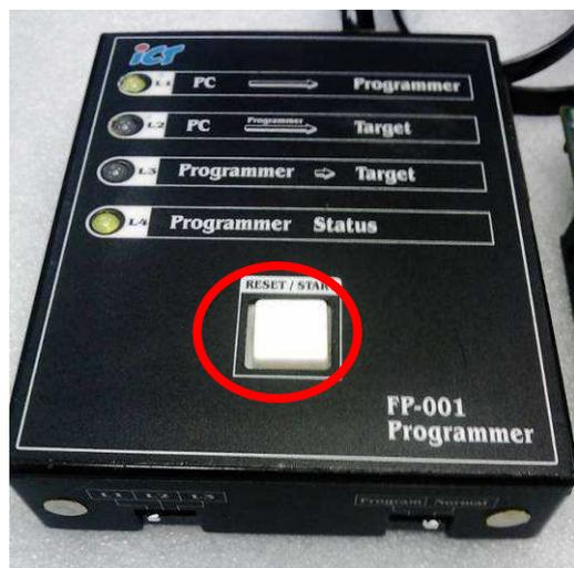
Step3. Switching to Program and then switching to L3.
