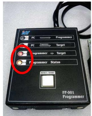
Step6. Press RESET/START button when L4 lighting in orange.
